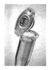
A needle placed through the thin membrane in the middle of the lid allows the aerosol-free removal of biohazardous substances
